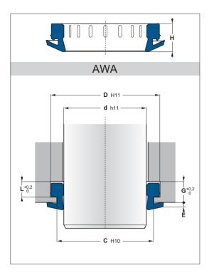
The function of **AWA** wiper is to prevent introduction of contamination into the system, to protect the guiding parts and to extend the service life of the rod seal. The wiper lip produces an effective cleaning action to avoid damage to all internal components.
