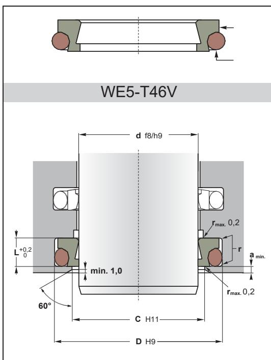
**WE5-T46V** Turcon® Excluder® 5 wiper has two different functions. It prevents introduction of dust, dirt and foreign matter into the system and on the medium side holds back the residual oil film passing the rod seal.
