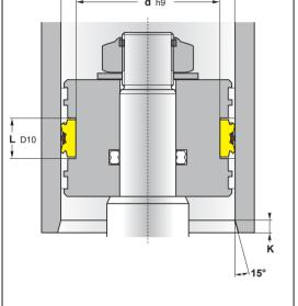
Hunger® TDMA tandem seal recommended for use where different fluids on each side are to be separated.
