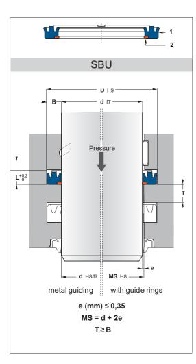
**SBU** U-ring is produced in a compact design which guarantees good functioning at low pressures and guarantees a particularly long service life. **SBU** is a single-acting rod seal. The semi-active back-up ring on the inner diameter prevents gap extrusion on the side facing away from the pressure.
