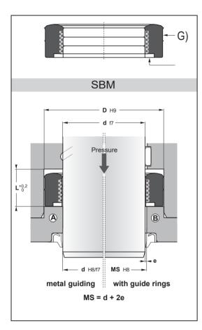
**SBM** compact rod seal has a great contact sealing surface in reinforced cotton fabric. To provide initial sealing under low pressure the inner surface has two sealing edges. Even with a worn piston rod the greater sealing surface continues to give good sealing.
