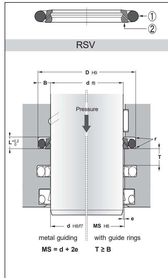
**RSV** Stepseal® V is based on the dynamic, unidirectional Stepseal® sealing concept. During the extending stroke of the rod, focusing of contact force on the unique Stepseal® sealing edge creates high local sealing pressure and limits the micro fluid film formation under the seal.
