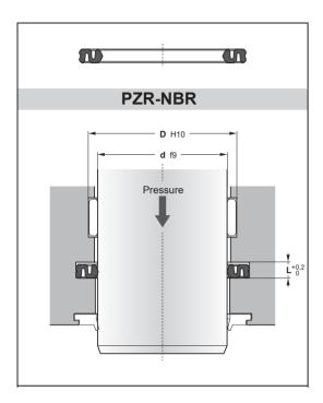
**PZR-NBR** rod seal has been designed for pneumatic cylinder applications. **PZR-NBR** can also be used for pneumatic valves.
