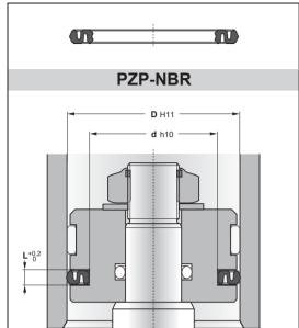
**PZP-NBR** piston seal has been designed for pneu-matic cylinder applications.
