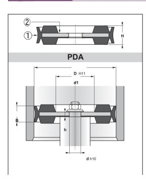
**PDA** double-acting is a complete pneumatic piston with a double cup seal and a vulcanised metal disc support.
