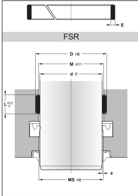
The **FSR** has been developed to substitute traditional bronze guides in hydraulic cylinders. They guide the rod and prevent metallic contact with the cylinder when radial forces act perpendicular to the direction of movement.
