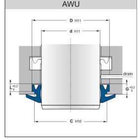
**AWU** wiper has two different functions. It prevents introduction of dust, dirt and foreign matter into the system and on the medium side retains the residual oil film from the extending piston rod.
