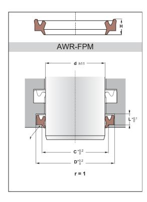
**AWR-FPM** wiper has two different functions. It prevents introduction of dust, dirt and foreign matter into the system and on the medium side retains the residual oil film from the extending piston rod.
