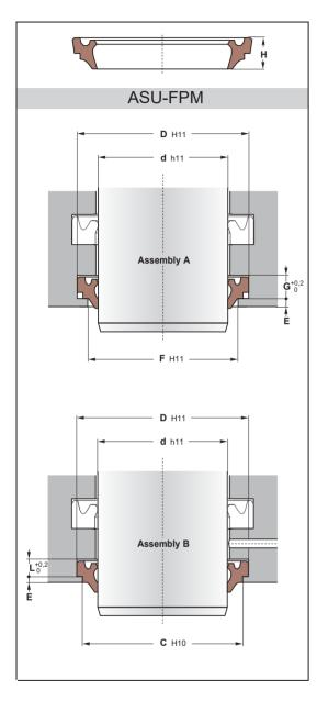
**ASU-FPM** wiper has two different functions. It prevents introduction of dust, dirt and foreign matter into the system and on the medium side retains the residual oil film from the extending piston rod.
