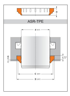
The function of **ASR-TPE** wiper is to prevent introduction of contamination into the system, to protect the guiding parts and to extend the service life of the rod seal. The wiper lip produces an effective cleaning action to avoid damage to all internal components.
