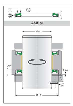
AMPM is a single-acting PU pin dust seal with two external metal cages for open groove assembly. The metal cages have to be pressed into the groove.
