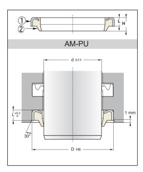
$\ensuremath{\mathsf{AM-PU}}$  is a single-acting  $\ensuremath{\mathsf{PU}}$  wiper with an external metal cage for open groove assembly. The metal cage
