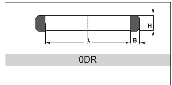
The **0DR** is designed to replace traditional seals in flange seal applications. With bidirectional sealing capability, the **0DR** provides exceptional sealing for static seal applications.
